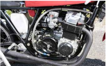
CB750F ('PVR 511R') purchased in April 2002. It is not known when it was last used. Noteworthy features include twin front disc brakes; 18" alloy wheel rims (Akront front, Morad rear); Avon racing tyres; an oil cooler; braided steel oil lines; Hagon shock absorbers; and Keihin CR carburettors. The machine comes with a substantial history file containing assorted correspondence, invoices and other paperwork (close inspection recommended).
