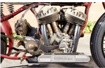
Today the reconstituted frame's main section and gas tank remain in their original, battle-worn paint, while the fork legs, rear frame section and fender have been repainted. Housed within the frame tubes – as it's been for the past 77 years – is the all-important factory Scout motor bearing its FCI-7 serial number and breathing though a Linkert carb set up to run on alcohol.
