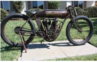
its as-raced condition. Amazingly, about 85% of the original parts remained. The engine was rebuilt to running condition, needing only a new set of pistons. A reproduction fuel tank, fork tubes, handlebars and rear stand were fashioned, carefully patina'd to match the frame's original faded red paint.
