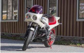
suspension and Brembo brakes. The tank, seat and fairing were specially customized, featuring twin head and twin taillights, and new 3-spoke, 17in wheels. The 6-into-1 exhaust system was handmade in stainless steel and the motor was modified to give 140 horsepower at the rear wheel but still maintain the original Honda drivability and reliability.
