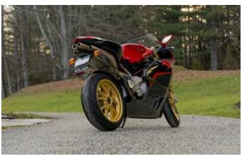
Only 300 limited edition Tamburini F4s were built for the world market. Each had a re-tuned 4-cylinder engine installed producing 173 horsepower, and included a magnesium swing arm and frame plates, a carbon fiber kit comprising air box, air ducts, tail fairing, front mudguard, side panels, and upper and lower chain guards, plus special graphics, an instrument panel with a stopwatch, and a gold serial number plate on the steering head.
