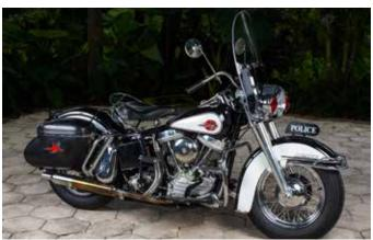
This 74 ci motorcycle is a basic FLH, meaning it has a hand shift, four speed transmission. There were three police option packages for 1960. FP-1 had the front fender mounted siren with hand control, speedometer hand control, oil filter and Deluxe solo saddle. FP-2 provided a foot control for the siren while the final option package FP-3 designated a rear mounted siren. With the sprung solo saddle, it was a comfortable ride.
