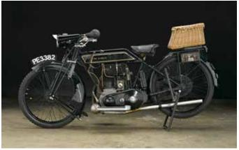
this tank is a piece of artwork to be appreciated like a Monet. Up front, a set of Druid forks cancel out the roughness of the roads with an acetylene lamp to light the way at night. This period British motorcycle used thumb levers to control the spark advance and throttle, unlike the twist grip throttles found on American motorcycles. The finish reflects the enjoyment of use and there is much original nickel plating on the motorcycle with original leather tool boxes.
