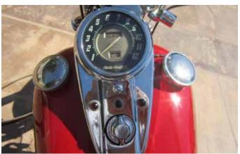
original zero miles Panhead speedometer that looks perfect on top of the tanks. Flanders risers and handlebars set atop the original, chromed forks. Other accessories include a cast aluminum spark plug holder, black solo leather seat, a Tombstone tail light and Cycle-Ray headlight wired to a 6 volt system.
